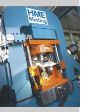
Above: Front view of the optional HME fast Hydraulic Tool Clamping System.
