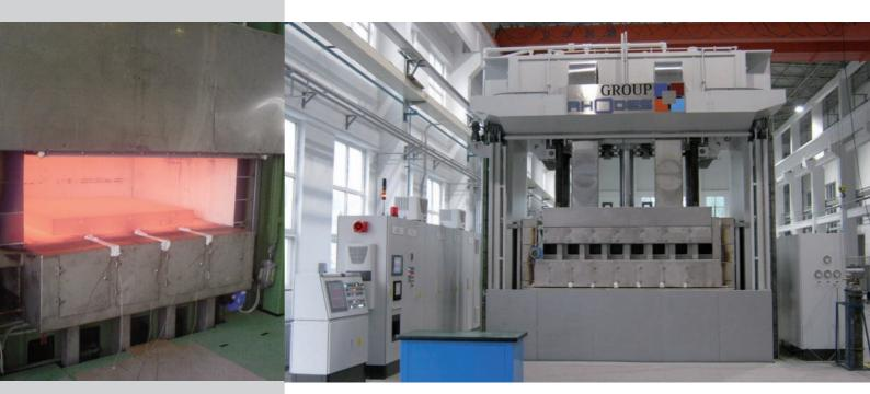
Main (right): 1400 tonne SPF/DB press complete with semi-automatic tool loading equipment
