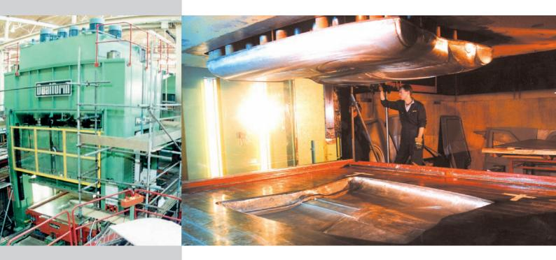
**Main right:** Top and bottom tools manufactured in the Dualform Model 9 press ready for pressing panels.
