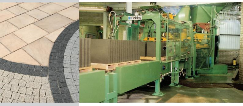
Main (right): Paving Slabs produced using a Fielding & Platt Wet-Mix Process
