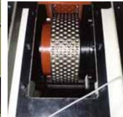
**Berry Refractories** manufacture a range of Compression Presses, in particular Roller Briquette Presses (left and above) used in the production of anthracite briquettes at rates of up to 15 tonnes per hour. Manufactured from coal, the anthracite briquettes are used as a form of smokeless fuel.
