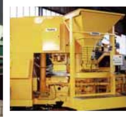
The **Fielding and Platt** range of concrete machinery is specifically designed for producing high quality concrete products by either the Semi-Dry Mix Process or Wet Mix Process. Ancillary products, such as Take-Off Edge Stacking Units (illustrated left) and automatic Mould Filling systems (above) are available to complement the full range of Fielding and Platt concrete presses.
