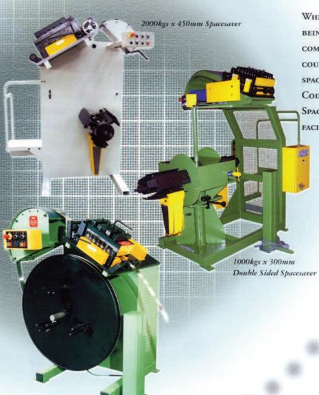
Where space is a problem and the material being processed is less than 2.5mm thick, a combined coilholder and straightener could be the solution. Designed to save space, there is no looping area between the Coilholder and the Straightener.
