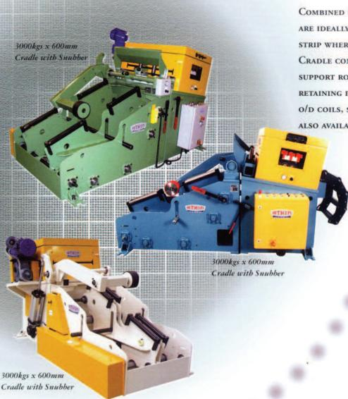
COMBINED COIL CRADLE AND STRAIGHTENERS ARE IDEALLY SUITED TO PROCESSING THICKER STRIP WHERE FLOOR SPACE IS LIMITED. THE CRADLE COMPRISES A FABRICATED FRAME WITH SUPPORT ROLLERS AND ADJUSTABLE SIDE RETAINING PLATES. SPECIAL FRAMES FOR 1600MM O/D COILS, SNUBBERS AND PRE-BEND UNITS ARE ALSO AVAILABLE.
