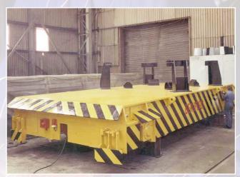
Customer: Avesta SMACC Project: 135 Tonne Capacity Scrap Basket Transfer Car
