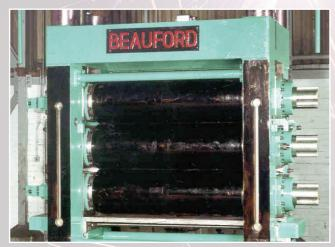
Customer: DSRM Project: 3 High Reversing Roughing Mill
