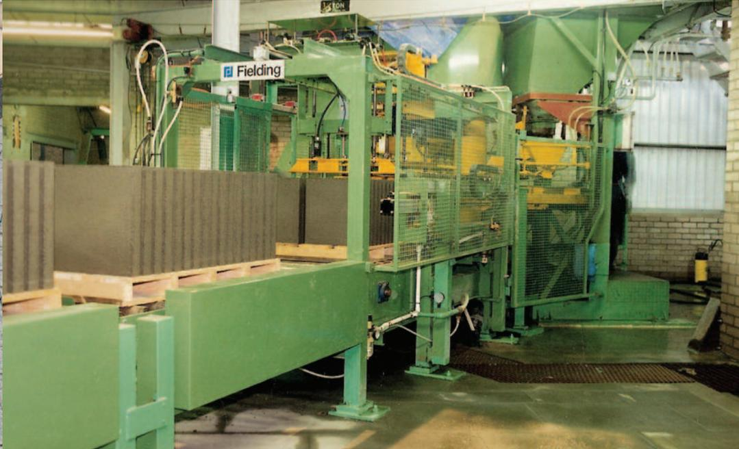
**Main (right):** Paving Slabs produced using a Fielding & Platt Wet-Mix Process
