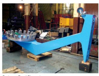
Customer: Royal Observatory Project: Telescope Bracket Use: Bracket for high powered telescope
