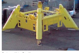
Customer: Vetco Gray Norway Project: Over Trawlable Structure Use: Oil and gas extraction from the seabed
